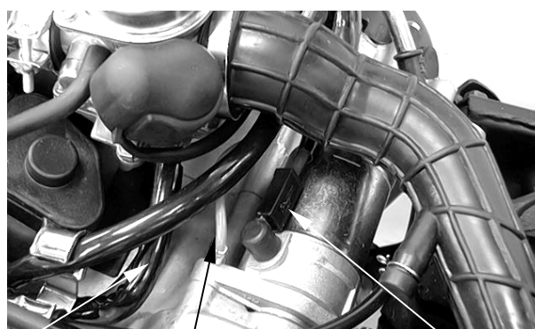
fuel tube Earthr Cable Starter Motor Cable
